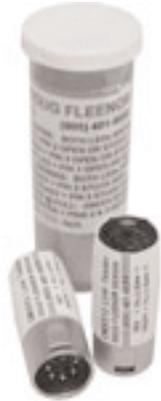
The DMX512 Line Tester instantly displays the presence of the +Data and -Data signals when plugged into a DMX control line or feed-through connector. Observing the indicators while fading all the dimmers from zero to full will detect if either line is stuck high. Swapped +Data and -Data lines can be determined by sending all dimmers to full.
